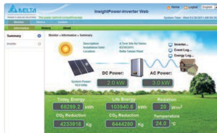
Solar system general information display
